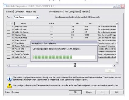
This indicates that the AOP is comparing the parameter data entered offline vs. the parameter data that is stored in the ArmorStart device. If any discrepancies are found between the parameters in the AOP and the parameters in the ArmorStart device, a window will pop-up, as shown below, asking you to decide which parameters you want to keep.
