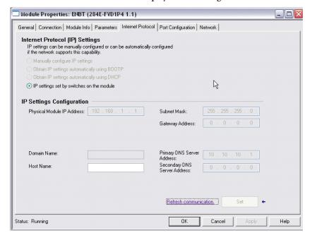
If the IP address was set up using the Rotary Network Address Switches, default settings for the IP would already be established and you will not be able to make any changes in this tab. In most cases, you would not need to make any changes in this tab and it only displays the current IP Settings Configuration.
