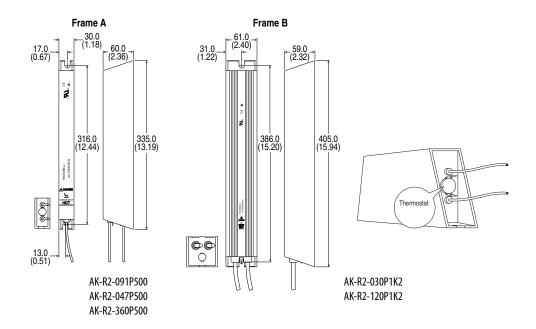
Recommended thermostat control wiring to prevent dynamic brake overheating.
