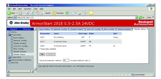
In the figure above the Starter Setup parameters are viewed. The user can view all parameters from this screen. To modify a parameter, the user clicks the "Edit" button.
