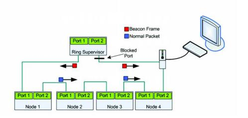
As shown in Figure 53, when a physical layer failure is detected the adjacent nodes to the fault generate a link status message that the ring supervisor acknowledges. The ring supervisor unblocks the port to allow communication. The neighboring nodes to the fault identify the fault and reconfigure themselves to support a linear topology. Now, both the ring supervisor and nodes are configured to support a linear topology.
