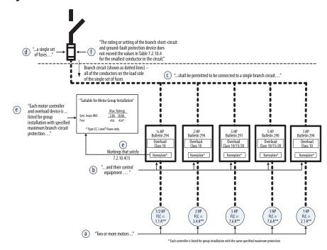
Figure 108 - ArmorStart LT NFPA 79 Multi-Motor Branch Circuit
