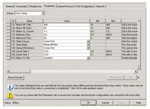
The parameters are divided into groups that are based on the type of ArmorStart device. By clicking in the Group pull-down menu, you can choose which parameter group is displayed. When the Parameters tab is selected, the tab defaults to the Drive Setup (Bulletin 284E) or Starter Setup (Bulletin 280E) groups depending on the ArmorStart selection. These Setup groups are the minimum required parameters to get the ArmorStart device running.
