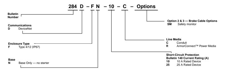
Table 61 - Bulletin 284E Base Module Renewal Part, IP67/Type 4/12, Up to 600V AC With Conduit Entrance
