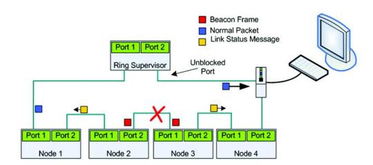
When the physical layer fault is corrected the supervisor will "hear" the beacon frame again on both ports. Once this is detected the ring supervisor re-establishes and configures the ring topology. All neighboring nodes detect this and reconfigure themselves back to ring. A DLR network is a single-fault tolerant network that is intended for the interconnection of automation devices.
