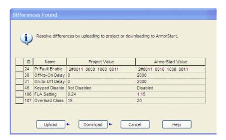
If you want to keep the parameters in the AOP, select Download. If you want to keep the parameters in the ArmorStart device, select Upload. Otherwise, select Cancel. Clicking Cancel locks the user out of viewing the values. If you are connected to a new ArmorStart device and you just created the ArmorStart object and have not made any changes in the parameters, the ArmorStart correlation should not find any discrepancy.
