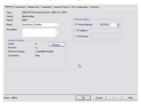
This tab allows you to name your module, which should be descriptive and representative of the module. The IP Address of the module must also be input so that communication can be established. The IP Address should be the one defined using the BootP/DHCP Server, the Rotary Network Address Switches or the ArmorStart internal web server.
