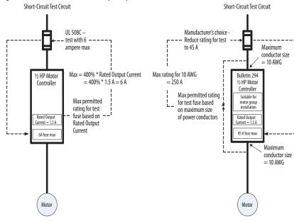
Figure 107 - UL508C Variable-Frequency AC Drive Motor Controller Evaluation
