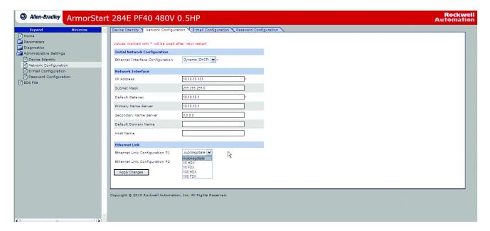
From this screen you can change the Ethernet Configuration. For example, in the above image the default IP address was changed from 192.168.1.1 to 10.10.10.101. To access the webpage after a power cycle, the new address must be used.
