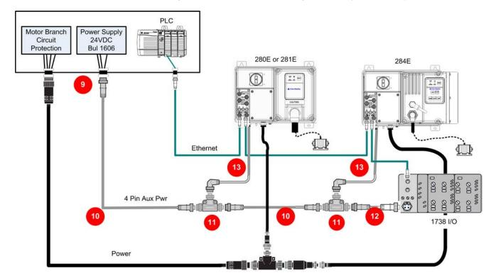
Figure 34 - Control Power Overview using 4-Pin Auxiliary Power Tee Adapter
