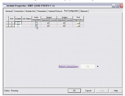
This tab is used to enable or disable a physical port in the module. The ports are normally in Auto Negotiate mode, which in general, is the recommended setting. Otherwise, you have to physically set the Speed or Duplex selection in this tab. It is important to note that although there are two physical ports, they act as one. Therefore, when you press either of the Port Diagnostic buttons, information coming from both of the physical ports is displayed.
