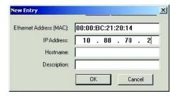
3. Enter the IP Address that you want to assign to the device, and click OK. The device is added to the Relation List, displaying the Ethernet Address (MAC) and corresponding IP Address, Hostname, and Description (if applicable).
