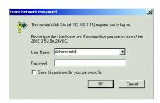
The user is prompted to enter the default user name (Administrator). There is no password set by default. The user is expected to change the user name (login) and password to avoid unauthorized access to the device configuration.
