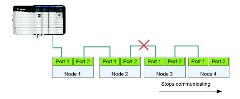
The EtherNet/IP embedded switch technology allows this topology to be implemented at the device level. No additional switches are required.
