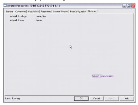
This tab displays information about the network configuration, such as the type of topology (linear or device level ring).
