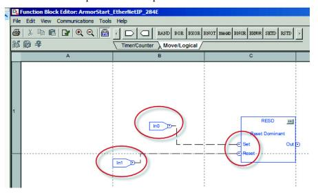
11. From the toolbar, Click the "Bit Output" button and select "Run Forward" from the hardware boolean tree. Run Forward is the relay controlling the coil of the contactor.
