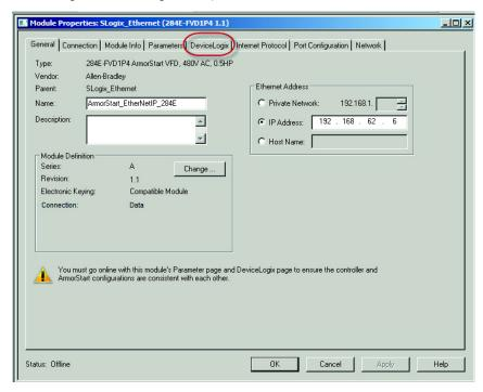
In addition to the actual programming, DeviceLogix can be configured to operate under specific situations. It is important to note that the DeviceLogix program only runs if the logic has been enabled. This can be done within the "Logic Editor." The operation configuration is accomplished by setting the "Network Override" and "Communication Override" parameters. The following information describes the varying levels of operation:
