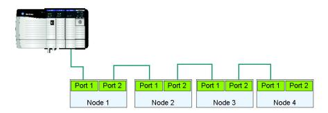
In this topology a communication issue in the media or device prevents nodes downstream from communicating.
