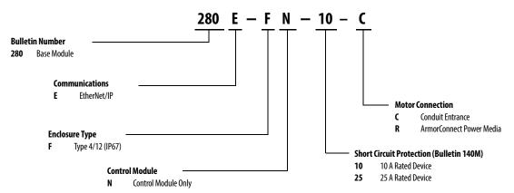
Table 57 - Bulletin 280E Full Voltage Starters and Bulletin 281E Reversing Starters – IP67/NEMA Type 4, with Conduit Entrance
