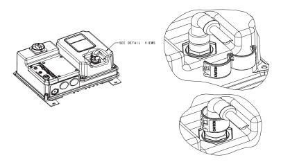
Figure 47 - Bulletin 284E Installation of Locking Clip
