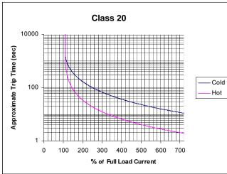
Note: For 280 and 281, if an overload fault occurs it may require 60 s or more before a fault reset is allowed. Refer to Overload Class Parameter 107, Thermo-Utilization parameter 105, and OL Reset Level parameter 108 to adjust the reset time.
