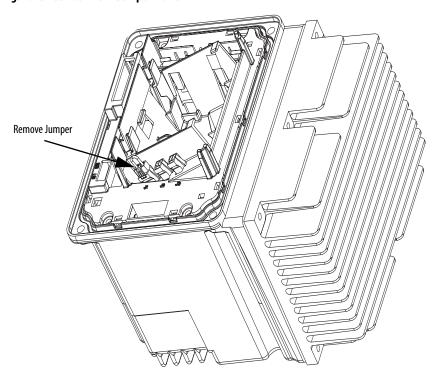
Figure 25 - Bulletin 284E Jumper Removal
