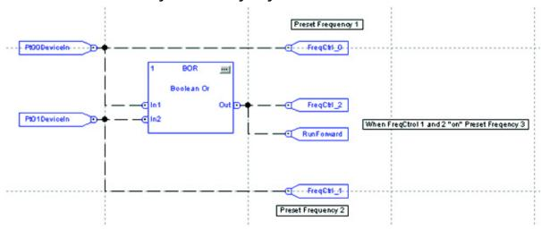
Once you exit the DeviceLogix editor, verify that the logic is "Enabled" otherwise the preset frequency control does not operate. See <u>Figure 118</u>.
