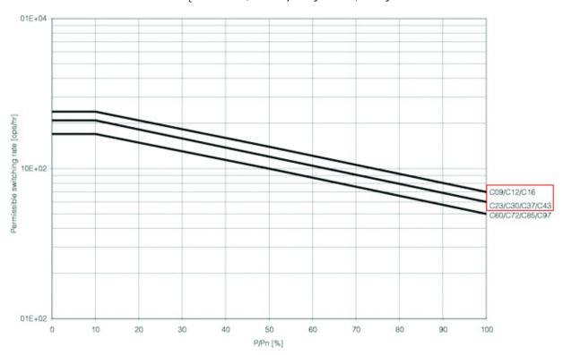
AC-4 Inching of squirrel-cage motors  $Ue=230\dots 460V, \, Starting \, time \, tA=0.25 \, s$
