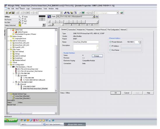
The screenshot above displays that the AOP has seven tabs that can be used to configure and/or monitor your ArmorStart selection. The following lists the tabs and whether they are editable or not, with the controller when OFFLINE, ONLINE, or both:
