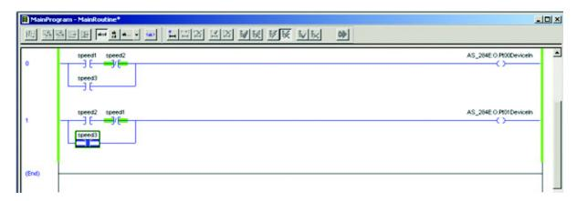
Download the finished program file to the PLC. In order for the parameters and DeviceLogix program to update in the device, verify the PLC is in program mode, and open the AOP for the Bulletin 284E.
