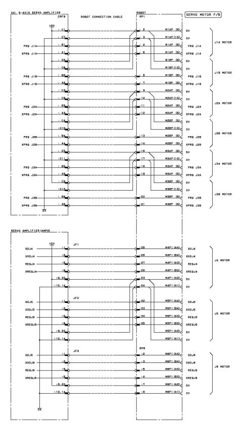
Fig.B (an) Pulsecoder Signal Connection Diagram (group6; M-430*i*A/2PH)
