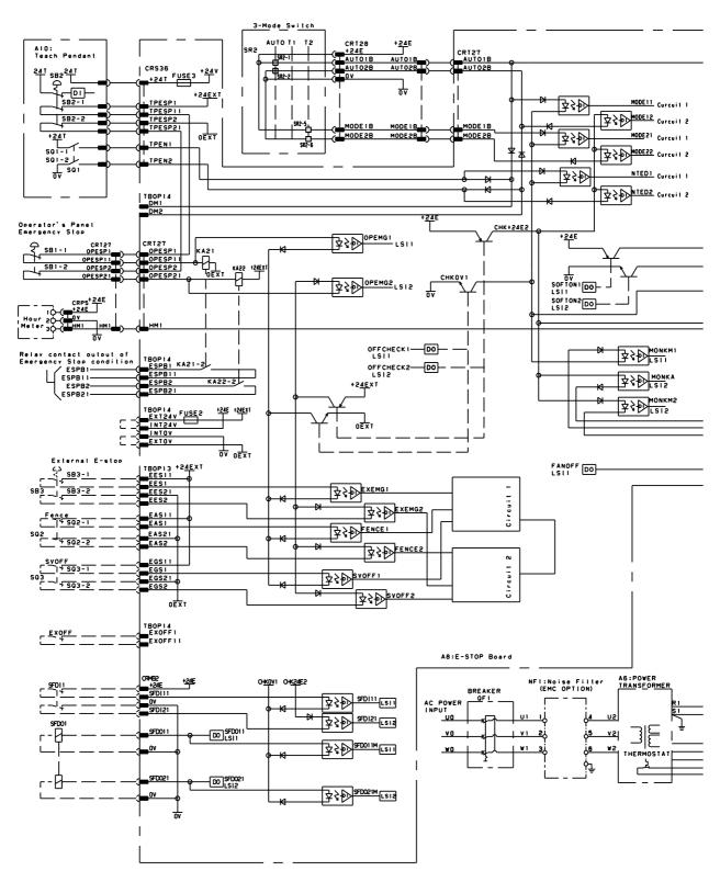
Fig.B (k) Emergency stop circuit connection diagram (A-cabinet/Resistor discharge)
