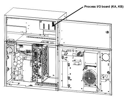
Fig.4(a) Locations of peripheral device interfaces (A-cabinet)
