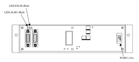
Fig.3.7.4 (c) LEDs on the process I/O board MB
