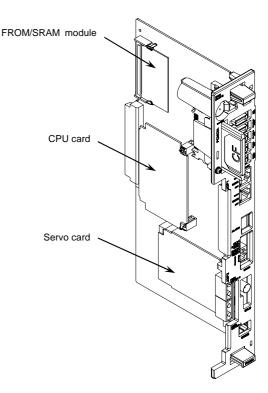
(R-30*i*B main board) (R-30*i*B Plus main board) Fig.8.2 (h) Locations of cards and modules
