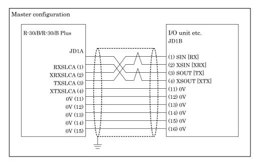
Fig.3.2.1.2 Cable connection diagram of the I/O Link cable when using JD1A connector
