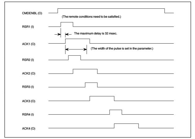
\* Other RSR signals can be accepted even when the ACK signal is being output.
