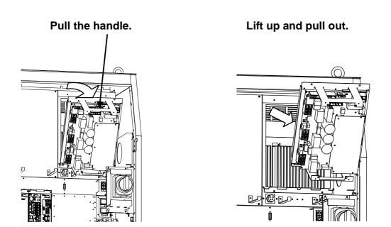
Fig.8.7(c) Replacing the servo amplifier (B-cabinet)
