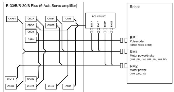
Fig.3.3.1 (c) Robot connection cable (Group4)
