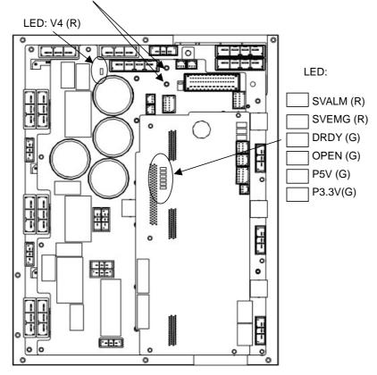
Fig.3.7.5 LEDs on the 6-Axis servo amplifier
