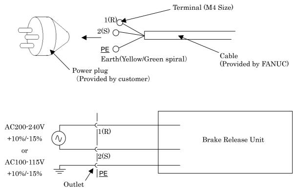
Fig.E.4 How to connect the plug to the power cable
