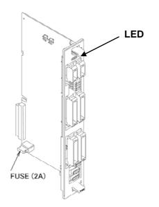
Fig.3.7.4 (a) LEDs on the Process I/O board JA/JB
