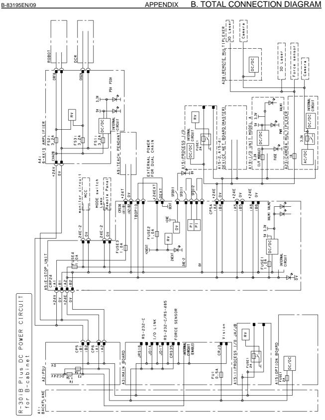
Fig.B (j) DC power line connection diagram (R-30iB Plus B-cabinet)
