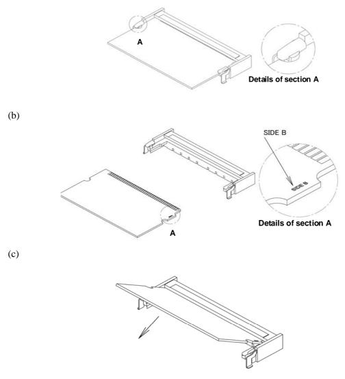
Fig.8.2 (g) Demounting/mounting a module
