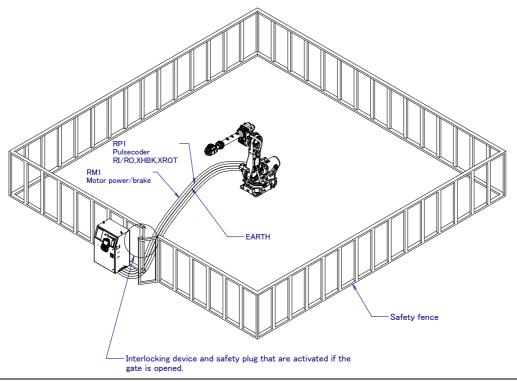
Fig. 3 (a) Safety fence and safety gate
