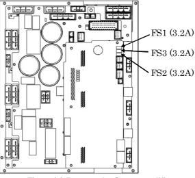
Fig.3.6(c) Fuse on the Servo amplifier
