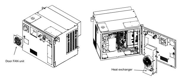
Fig.8.11.1 Replacing the heat exchanger and door fan unit (A-cabinet)
