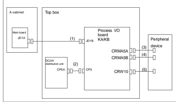
Fig.4.1.4 Block diagram of the process I/O board KA/KB
