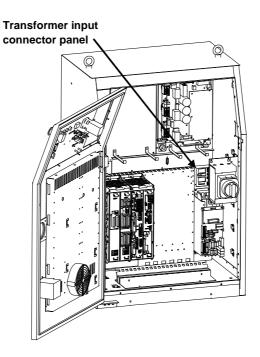
(2) Remove the rear panel. Remove (8)-M4 screws.
