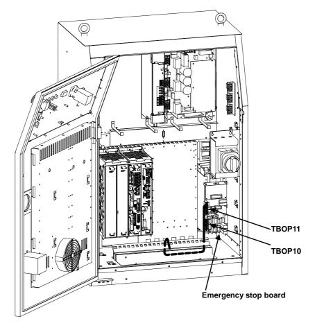
(B-cabinet) Fig.3.3.4 (a) Connection of the external power supply ON/OFF switch
