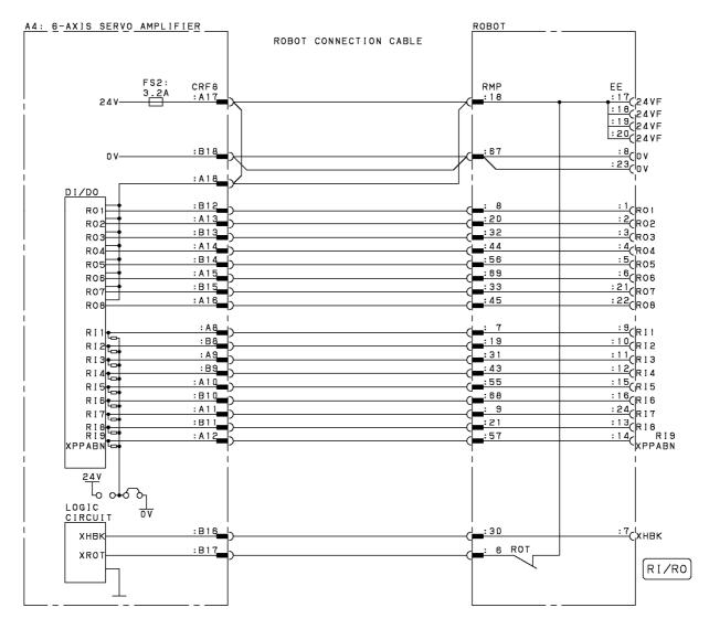
Fig.B (ai) RI/RO Connection Diagram (Group8; ARC Mate 100*i*C, ARC Mate 120*i*C)
