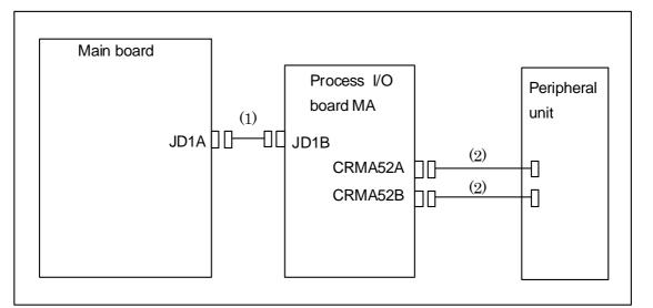
Fig.4.1.2 Block diagram of the process I/O MA
