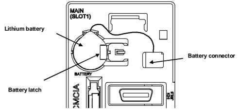
Fig.8.12.1 Replacing the lithium battery
