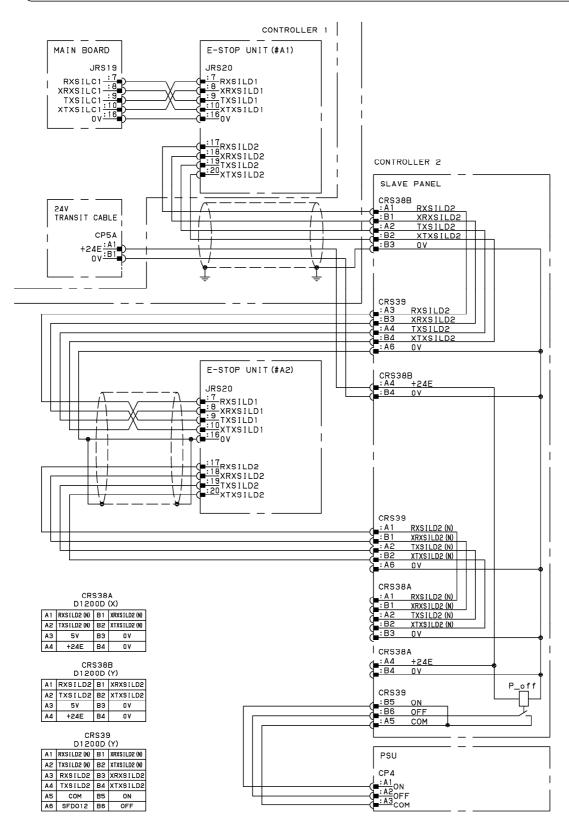
Fig.G.7(m) Connection between controller 1 and 2 (A-cabinet)
