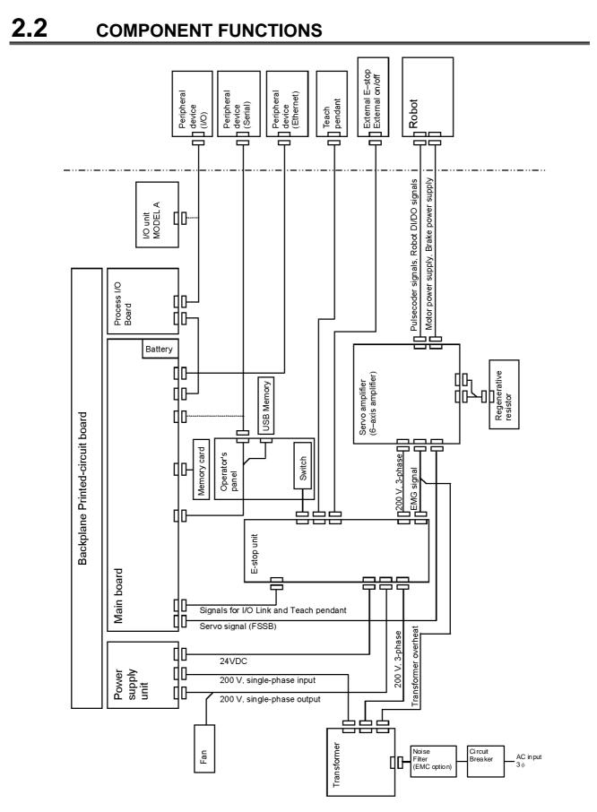
Fig.2.2 Block diagram of the R-30*i*B/R-30*i*B Plus
