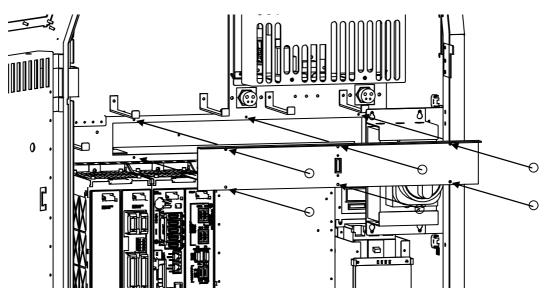
(Replacing the External Fan Unit)
