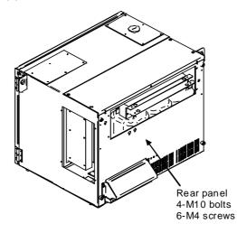
(5) Remove (4)-screws from the transformer input connector panel, and remove the (2)-M6 screws at the foot of the transformer. Then replace the transformer.
