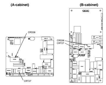
(Emergency stop board/A-cabinet) (Emergency stop board/B-cabinet) Fig.3.5 (a) SRVO-001 Operator panel E-stop
