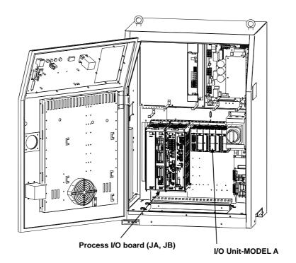
Fig.4(b) Locations of peripheral device interfaces (B-cabinet)
