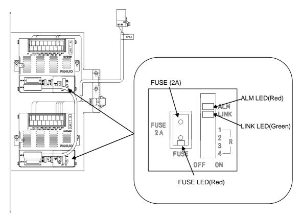
Fig.3.7.7 LEDs on the sensor I/F unit for CR-35iA
