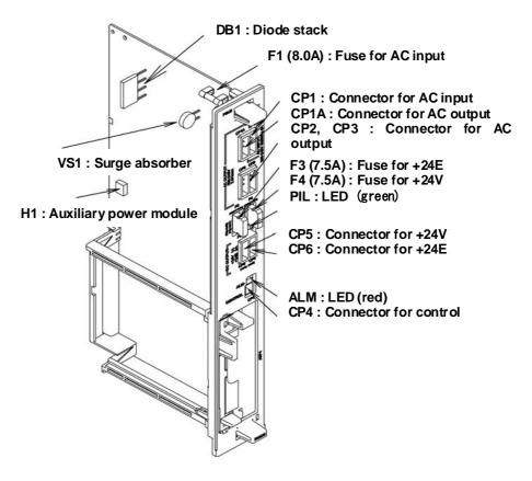
Fig.6.3 Interface of the power supply unit
