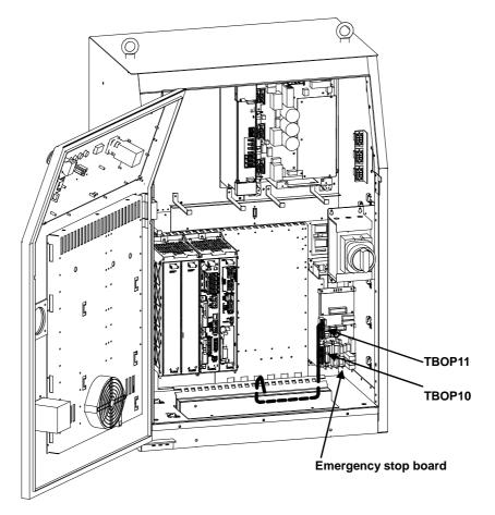
(B-cabinet) Fig.3.3.5 (a) Connecting the external emergency stop
