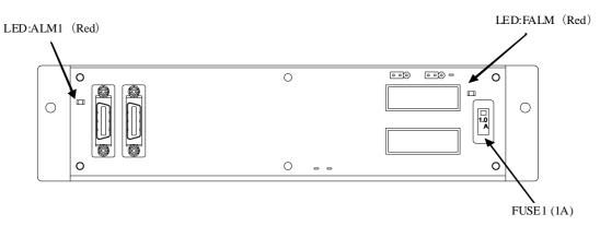
Fig.3.7.4 (b) LEDs on the process I/O board MA
