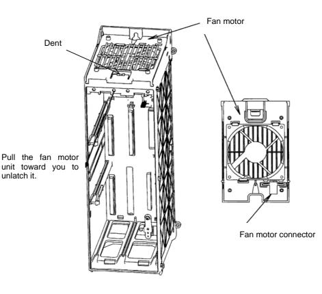
Fig.8.10 Replacing the control section fan motor
