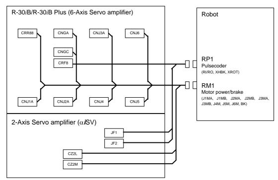
Fig.3.3.1 (e) Robot connection cable (Group6)
