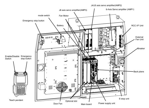
Fig.2.1 (f) R-30*i*B/R-30*i*B Plus B-cabinet interior (Front) (M-900*i*A/400L, M-900*i*A/600, M-900*i*B/700, M-900*i*B/400L)
