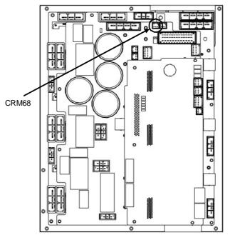
Fig.3.3.8 6-axis servo amplifier
