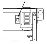
Fig.8.11.2 Replacing rear fan unit (A-cabinet)
