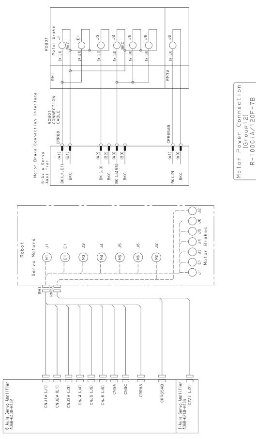
Fig.B (ae) Motor Power Connection (Group 12) R-1000iA/120F-7B
