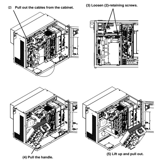
Fig.8.7(a) Replacing the servo amplifier (A-cabinet)
