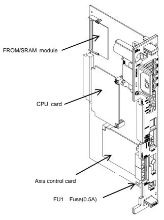
Fig.3.6(b) R-30iB Plus Main board
