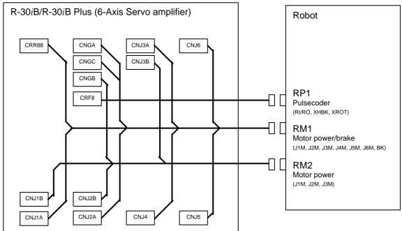
Fig.3.3.1 (b) Robot connection cable (Group3)
