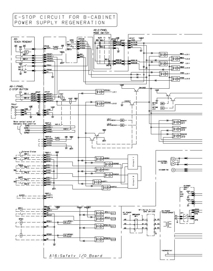
Fig.B (n) Emergency stop circuit connection diagram (B-cabinet/Power supply regeneration)
