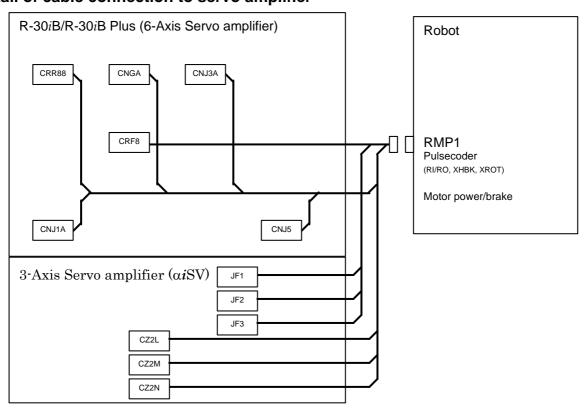
Fig.3.3.1 (f) Robot connection cable (Group7)
