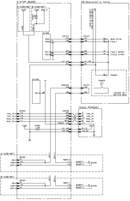
Fig.B (s) Operator's panel connection diagram
