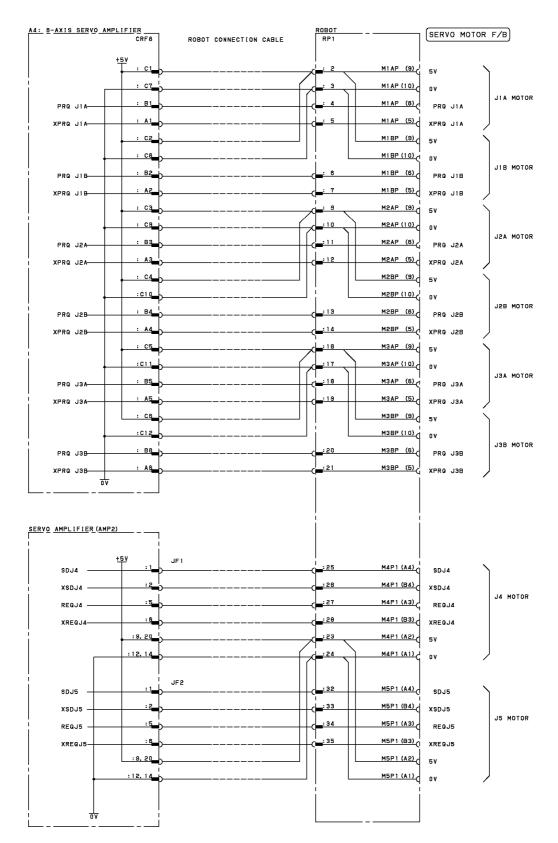
Fig.B (am) Pulsecoder Signal Connection Diagram (group6; excluding M-430*i*A/2PH)
