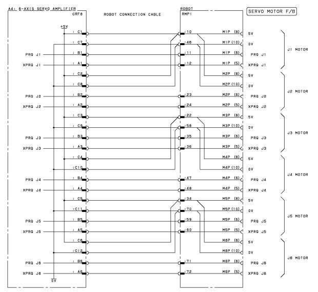
Fig.B (ap) Pulsecoder Signal Connection Diagram (Group8; ARC Mate 100*i*C, ARC Mate 120*i*C)
