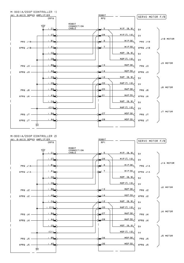
Fig.G.7(r) Pulsecoder signal connection diagram (Group 9:M-900*i*A/200P)
