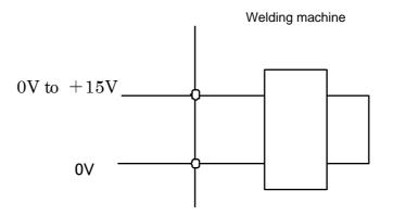
(b) Caution for use Input impedance:  $3.3k\Omega$  or higher Install a high-frequency filter.
