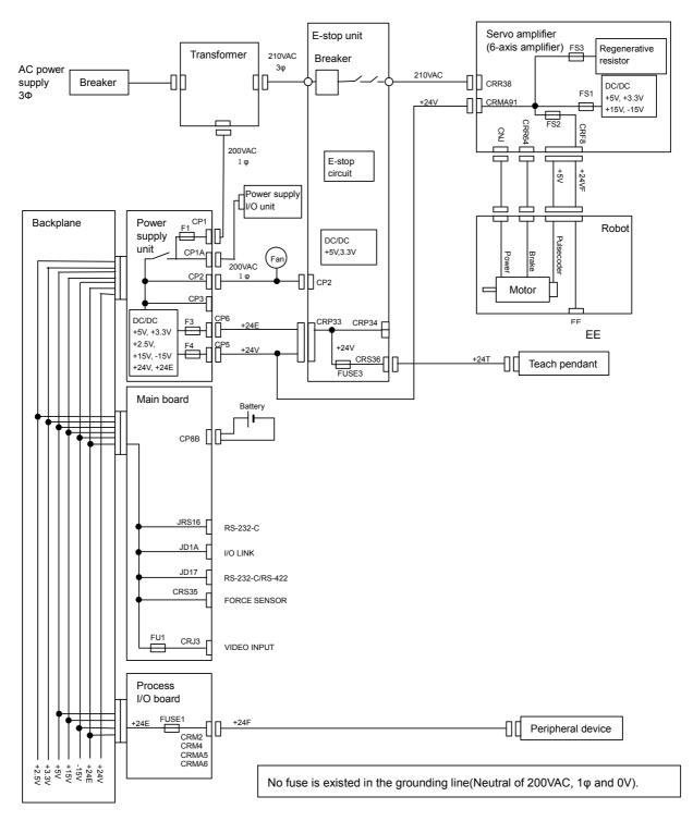
Fig.6.1 (b) Block diagram of the power supply (R-30*i*B Plus)
