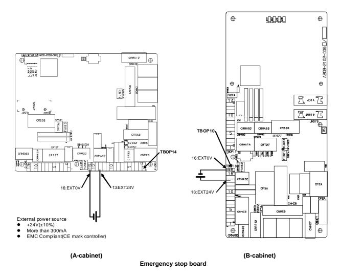
The relays for the emergency stop input and output can be separated from the controller's power. Please connect the external +24V instead of the internal +24V, if the emergency stop output must not affect the controller's power.
