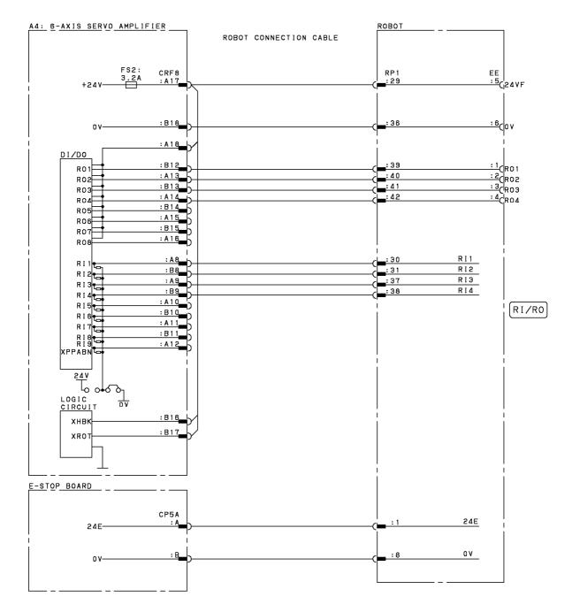
Fig.B (ag) RI/RO Connection Diagram (Group6; M-430iA/2PH,4FH)
