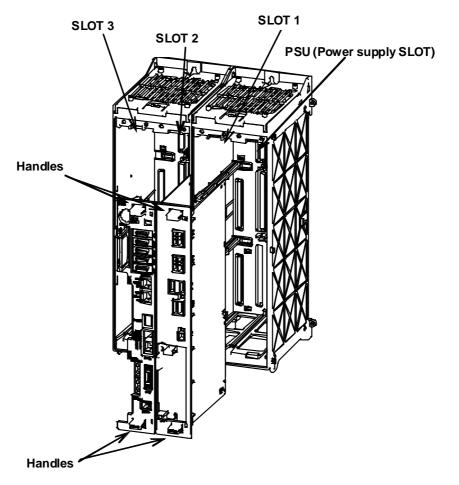
Fig.8.1.2 (b) Replacing the power unit and printed-circuit boards on the backplane
