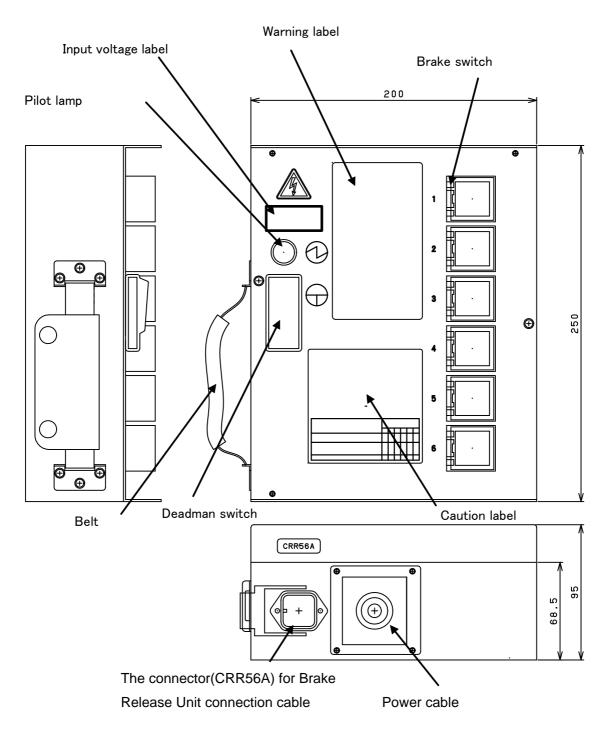
Fig.E.5 (a) Dimension of brake release unit (Front view)
