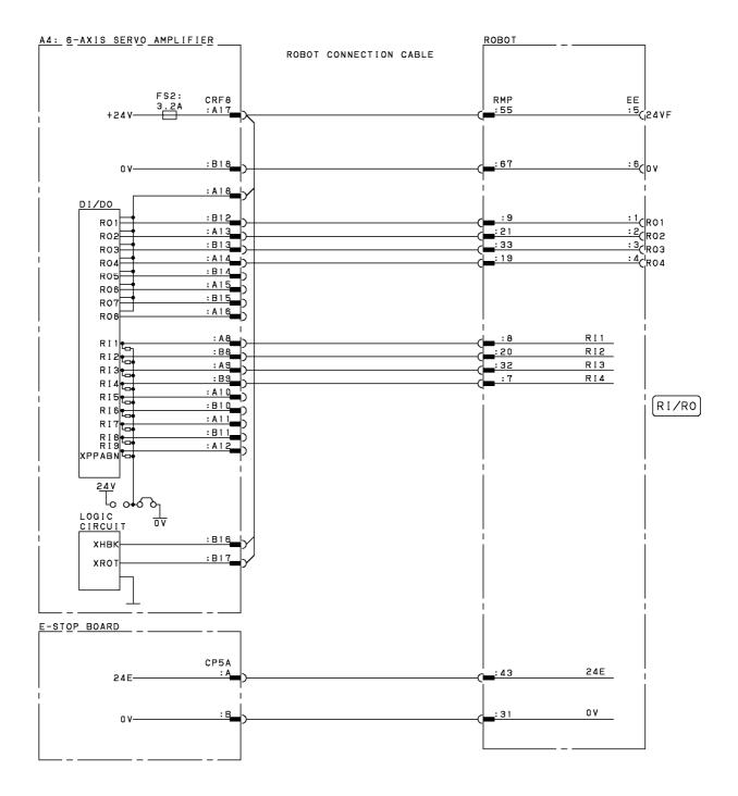
Fig.B (ah) RI/RO Connection Diagram (Group7; M-430*i*A/2P)
