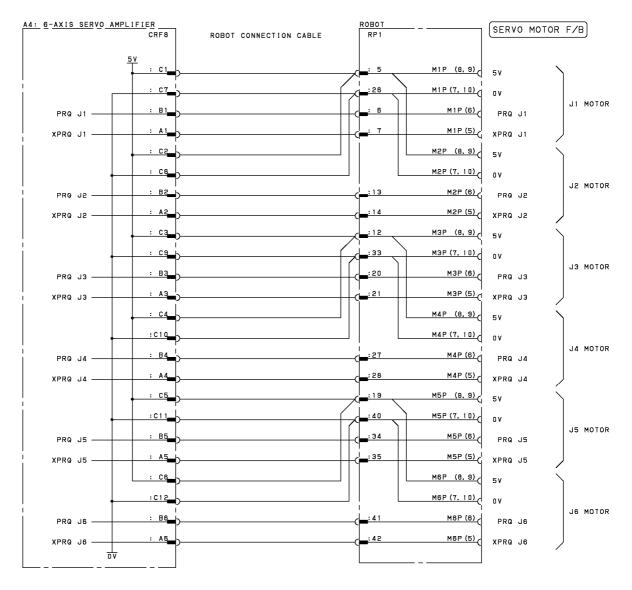
Fig.B (ak) Pulsecoder signal connection diagram (Group1 to 4, 11)
