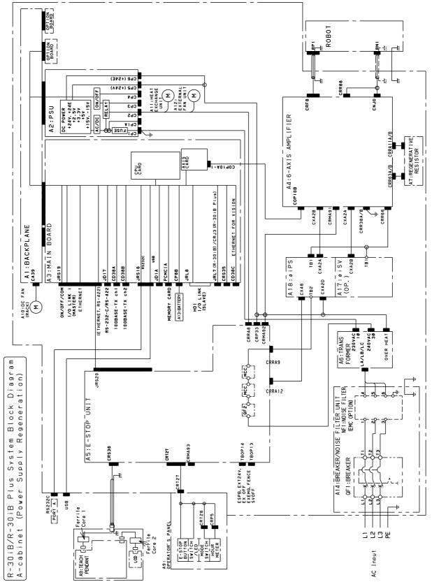
Fig.B (b) System block diagram (A-cabinet / Power supply regeneration)
