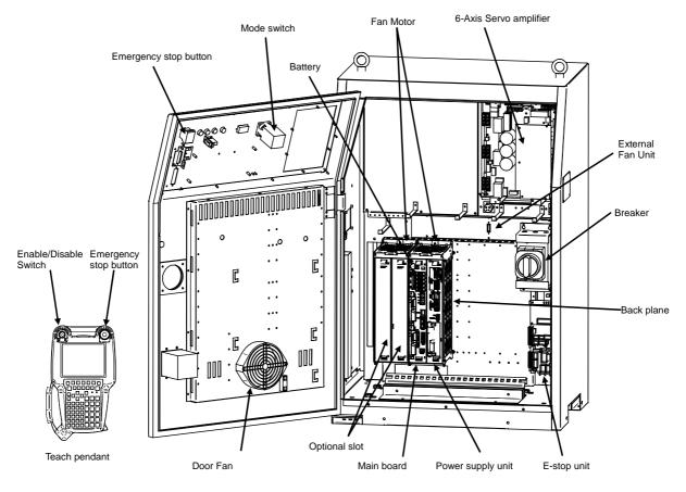
Fig.2.1 (e) R-30*i*B/R-30*i*B Plus B-cabinet interior (Front)
