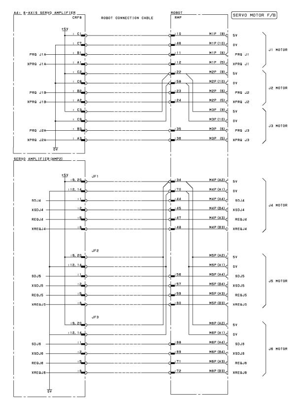
Fig.B (ao) Pulsecoder Signal Connection Diagram (Group7; M-430iA/2P)
