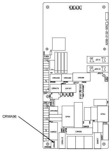
Emergency stop board (B-cabinet) Fig.3.3.6 Connecting the NTED Signal (B-cabinet)
