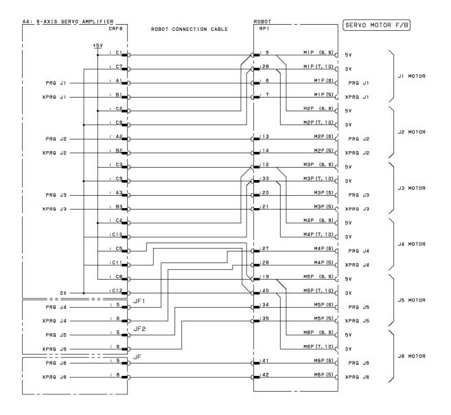
Fig.B (al) Pulsecoder Signal Connection Diagram (Group5; M-900*i*A/400L,600,M-900*i*B/400L,700)
