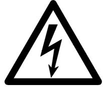
Fig.8 (c) High-voltage warning label
