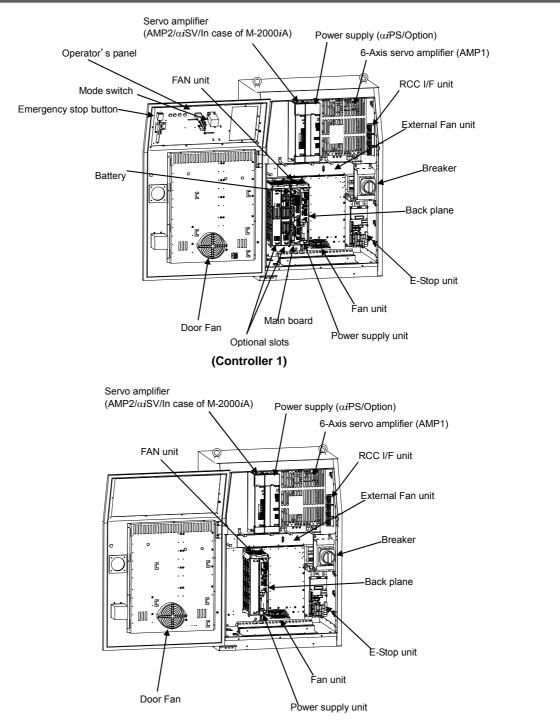
(Controller 2) Fig.G.1(a) M-900*i*A/200P, M-2000*i*A CONTROLLER (B-cabinet)
