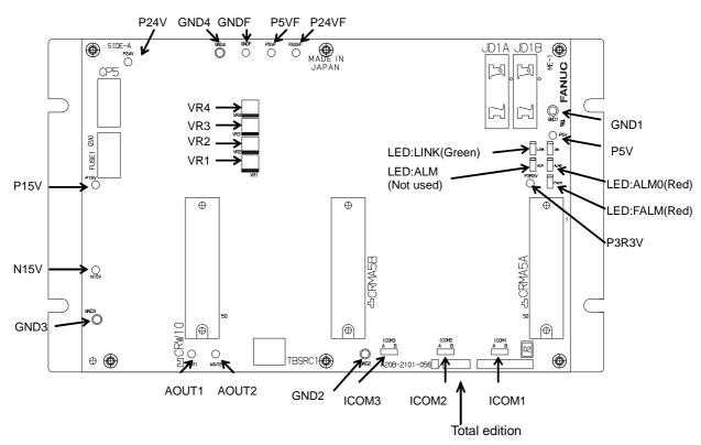
Fig.4.9 (b) Process I/O Board KB (Total edition 03B or later)
