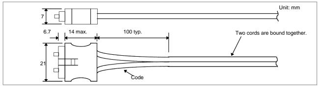
Fig.D (c) External dimensions of internal optical cable Unit: mm
