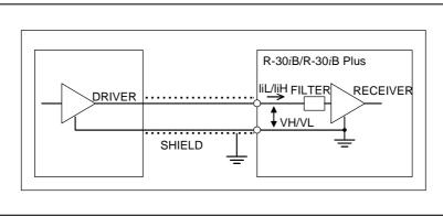
Absolute maximum rating Input voltage range Vin: -3.6 to +10 V Input characteristics
