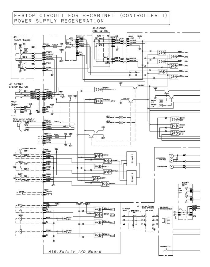
Fig.G.7(k) Emergency circuit connection diagram (B-cabinet/Power supply regeneration/Controller 1)
