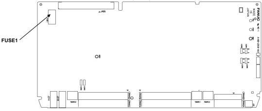
Fig.3.6 (e) Fuse on the Process I/O board JA,JB
