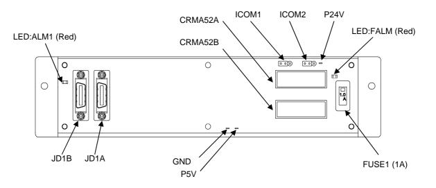
Fig.4.6 (a) Process I/O Board MA (Total edition 02A or earlier)
