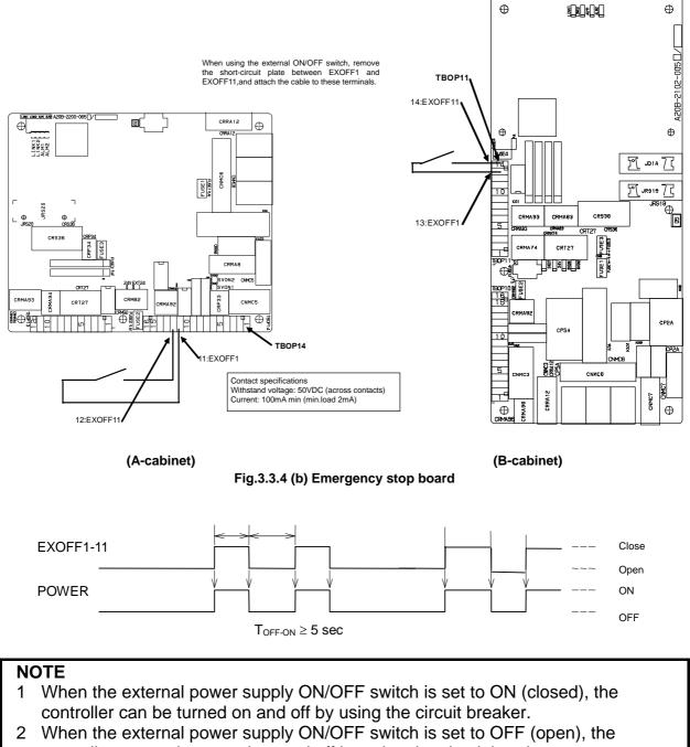
controller cannot be turned on and off by using the circuit breaker.
