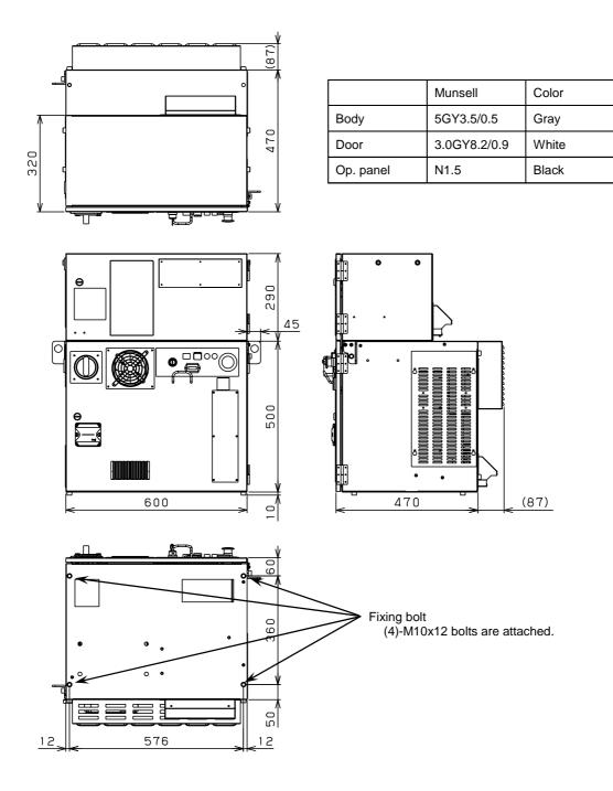
Fig.5.2.1(a2) External dimensions (A-cabinet with Top box)
