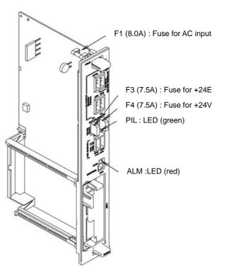
Fig.3.7.2 LEDs on the power supply unit
