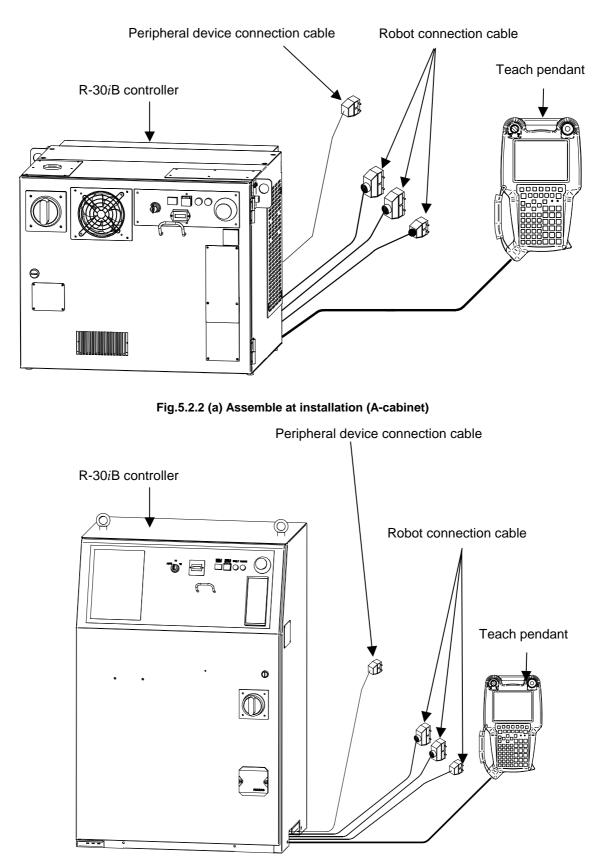
Fig.5.2.2 (b) Assemble at installation (B-cabinet)
