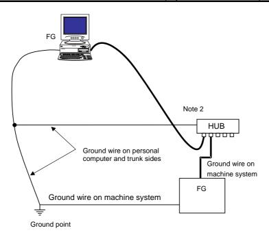
Wiring on a single ground point
