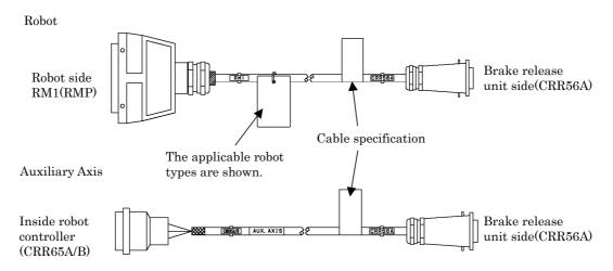
Fig.E.2 Brake release unit connection cable
