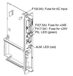
Fig.3.6(a) Fuse on the Power supply unit
