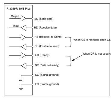
Generally signals as follows are used in RS232C interface.
