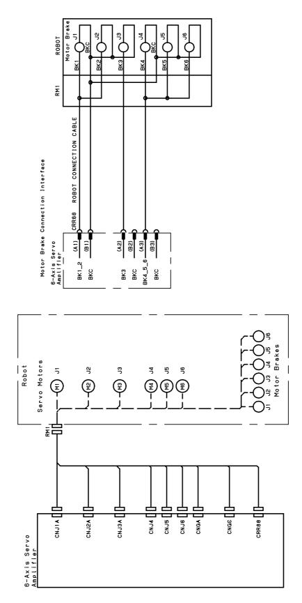
Fig.B (v) Motor power connection (Group1, Group11) Group1: R-2000*i*B(except /200T/220U/220US), R-2000*i*C(except /210L/270F), R-1000*i*A(except /120iF-7B), M-710*i*C,M-420*i*A,M-421*i*A Group11: M-2*i*A,M-3*i*A
