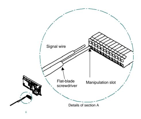
CONNECTIONS 3. ELECTRICAL CONNECTIONS
