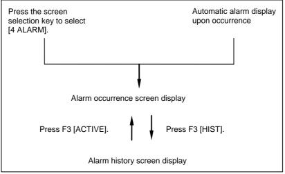
Fig.3.2 Alarm screen and alarm history screen display procedure
