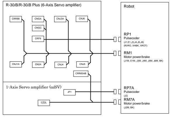
Fig.3.3.1 (h) Robot connection cable (Group12)
