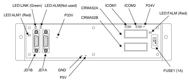
Fig.4.6 (b) Process I/O Board MA (Total edition 04B or later)
