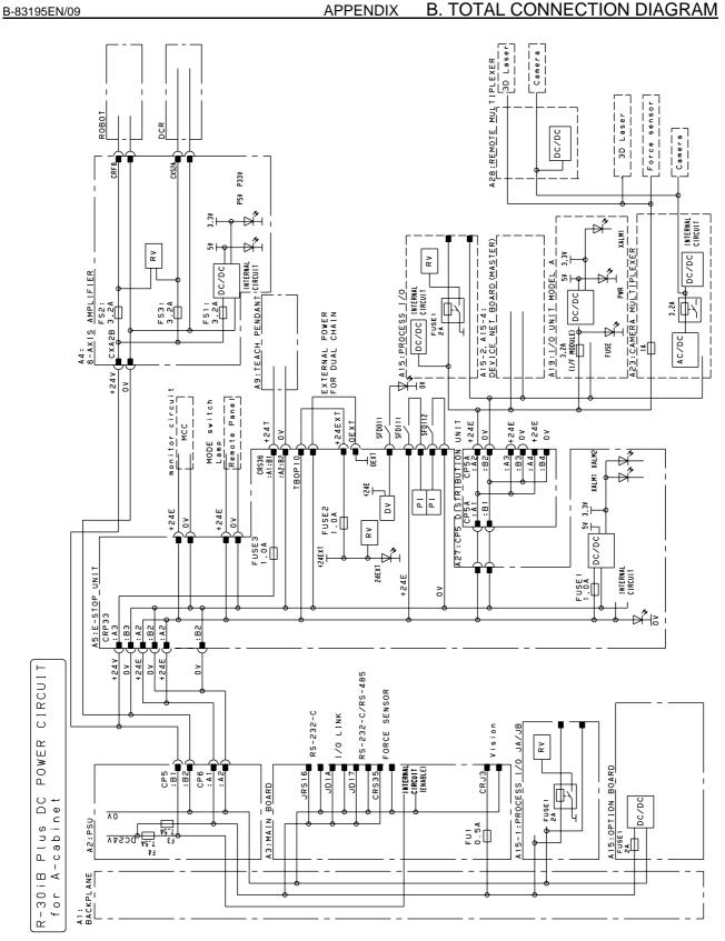
Fig.B (h) DC power line connection diagram (R-30iB Plus A-cabinet)
