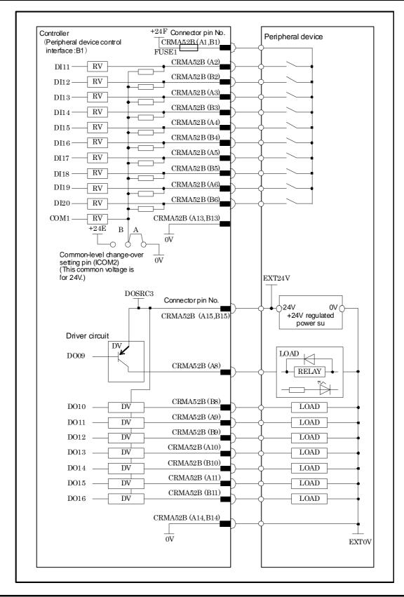
**NOTE** In this diagram, common voltage of input device is +24V.
