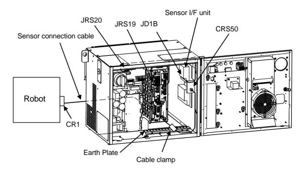
Fig. 4.11 Connecting the sensor connection cable
