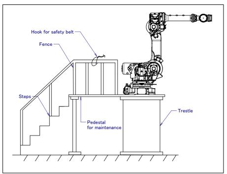
Fig. 3 (c) Pedestal for maintenance
