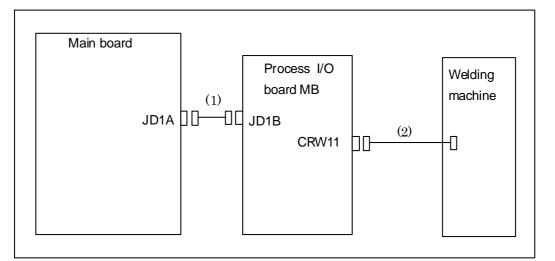
Fig.4.1.3 Block diagram of the process I/O MB
