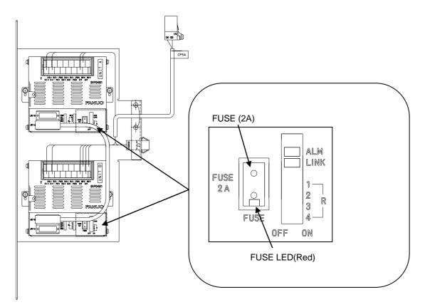
Fig.3.6 (h) Fuse on sensor I/F unit for CR-35*i*A
