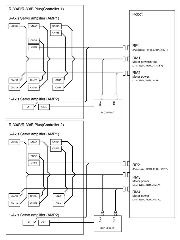
Fig.G.4(b) Robot connection cable (Group10: M-2000*i*A)
