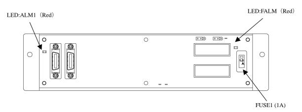
Fig.3.6 (f) Fuse on the process I/O board MA
