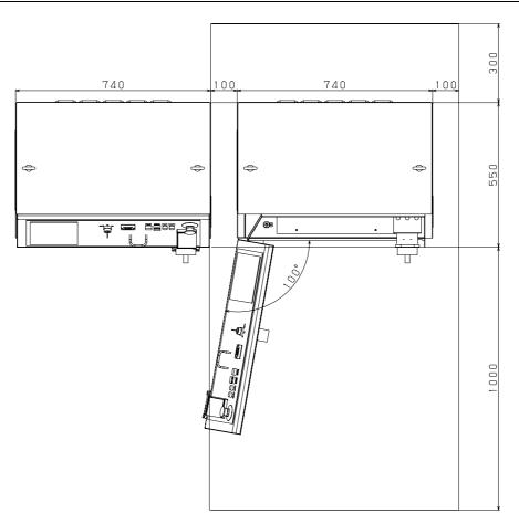
Fig.5.2.1 (e) Installation dimensions (B-cabinet)
