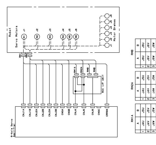
Fig.B (y) Motor power connection (Group4) M-900*i*A/150P,260L,350
