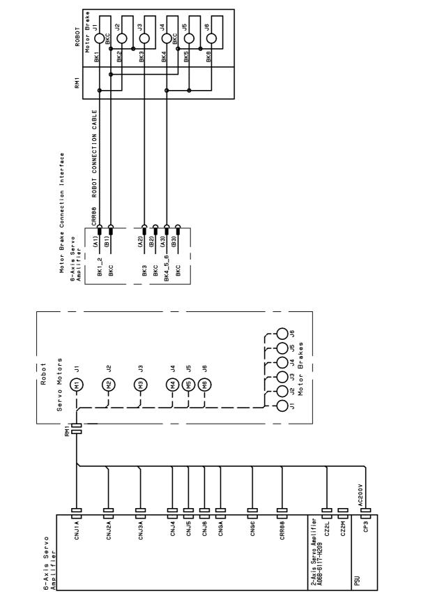
Fig.B (aa) Motor Power Connection (group6-1) M-430*i*A/4FH
