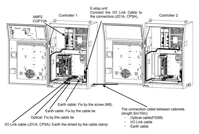
Fig.G.3 Installing the connection cable between cabinets
