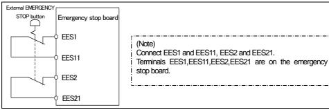
Fig. 3.1 Connection Diagram for External Emergency Stop Button
