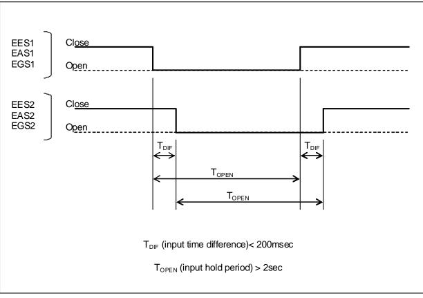
Fig.3.3.5(c) Input timing of duplicate safety signals
