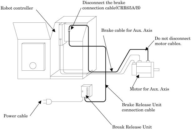
Fig.E.3.2 How to connect brake release unit (In case of operating to the Aux. Axis)
