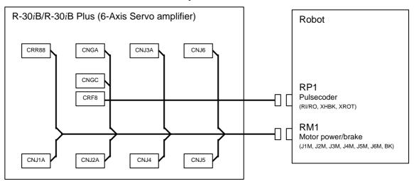
Fig.3.3.1 (a) Robot connection cable (Group1, Group2, Group11)
