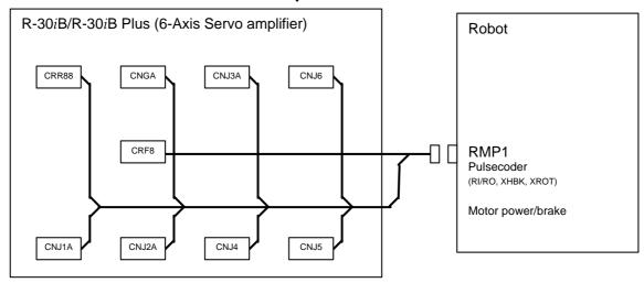
Fig.3.3.1 (g) Robot connection cable (Group8)
