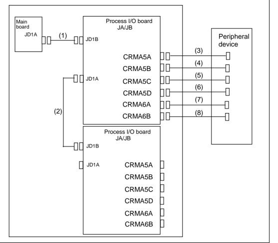
Fig.4.1.1 Block diagram of the process I/O board JA/JB
