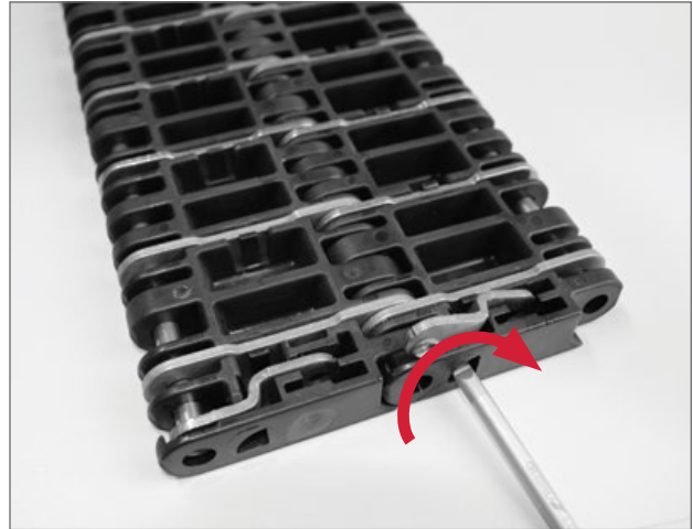
Twist screwdriver 90 degrees clockwise to open pin retention
