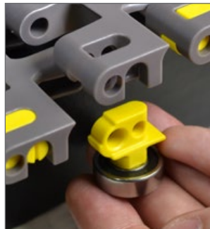
Attachment can be removed from bottom of chain
