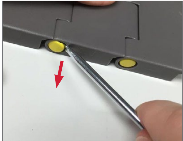
Disassembly — Insert the screwdriver under the plug to remove it
