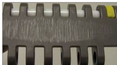
Scalloping to top of chain from stuck return rollers
