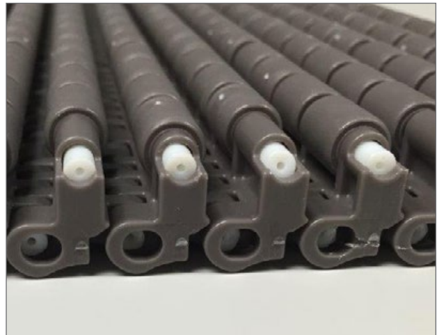
Assembly — Reinsert pin
