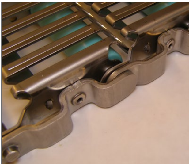
Pin retention clips are riveted to the side of the chain
