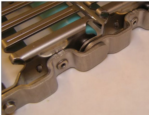
Chain with correctly installed pin retention
